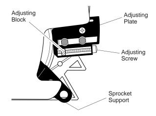
Figure 4 - Part Locations For Assembling Guide Bar
